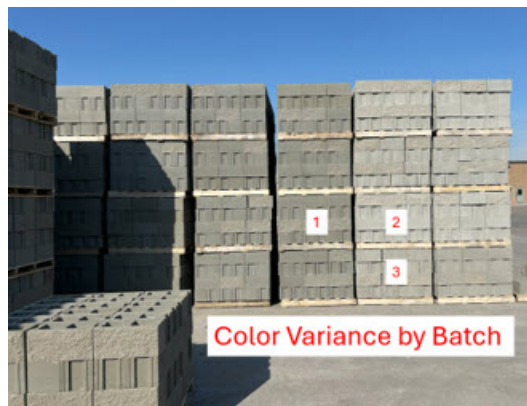
Inconsistent curing conditions can lead to unfortunate results.
