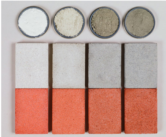
Note the effect of cement color on mortar samples. Lighter color cements produce brighter colors.
