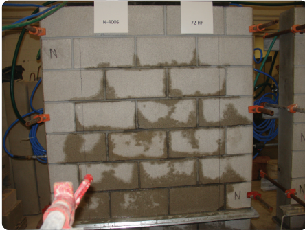
Untreated concrete masonry test wall (ASTM E514) after 72 hours
