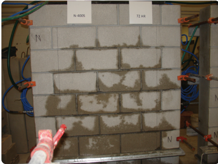
Untreated Wall after ASTM E514 Test
